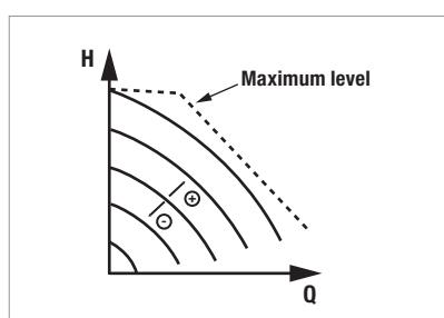
In this control mode, the circulator works on characteristic curves at constant speed. The performance curve is selected by setting rpm by means of a percentage factor. The value 100% indicates the maximum limit curve. Actual rpm may depend on the power and differential pressure limitations of your circulator model. Rpm can be set via the display or with a 0-10V external signal.
